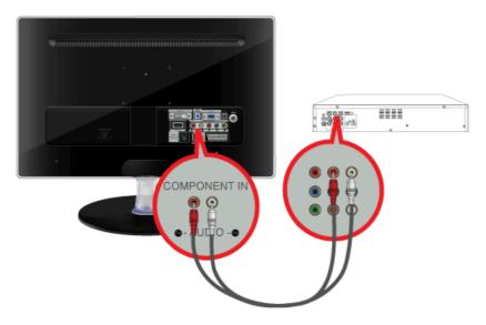
2. Connect the audio port of the AV device (DVD/VCR/Cable/Satellite box) to the [COMPONENT IN [R-AUDIO-L]] port of the monitor.
